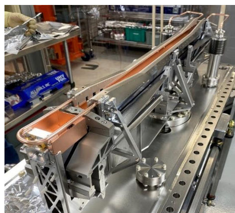
Prototype collimating mirror that employs a Gallium-Indium trough and a tuned conduction heat exchanger. Incorporating this new design into older beam lines will greatly improve performance of beam lines on high-power wiggler sources.
