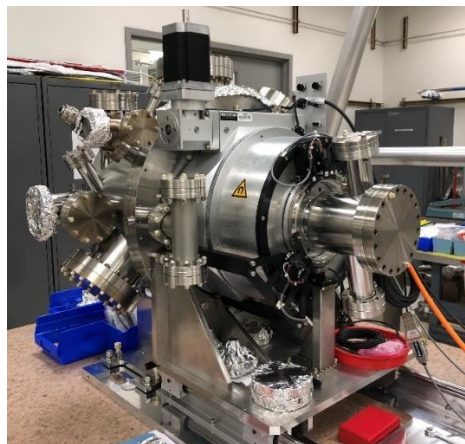
Fast-scanning monochromator designed for operando chemical catalysis science.
